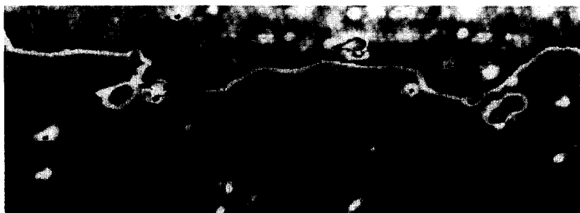
Fig. 9. Atomically resolved image of the border between the adlayer and the clean aluminum surface. 198 \text{ \AA} \times 82 \text{ \AA} , I = 0.3 \text{ nA} , V = -1.5 \text{ V} , T_{\text{ads}} = 350 \text{ K} , 6 \text{ L H}_2\text{S} .
