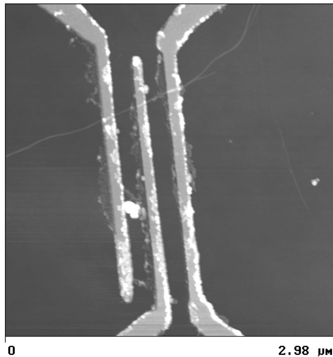
FIGURE 4.16. Re-electrode structure connecting a SWNT bundles. The height of the Re layer is about 25 nm. At the edges and on the metal lift-off, residues are clearly observable, as Re is much more ductile than, for example, Au or AuPd. The middle and the outside left electrode are short-circuited by lift-off residues.
