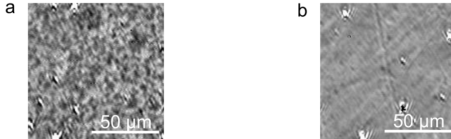
Figure 5.7: Kerr microscope image of Fe films with constant thickness grown at 130 K, shown after CO exposure. a: Perpendicular domain state of 3 ML Fe film after dosage of 12 L CO. b: Vanishing of the perpendicular domain structure after the same dosage of CO. The film has a thickness of 4.2 ML.
