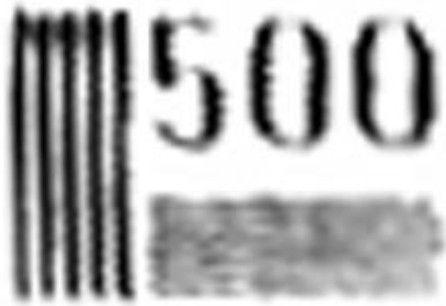
Figure 2.16: Optical grid with a spacing of 2 \mu\text{m} between two grid lines. Slightly reduced resolution in one direction is visible.
