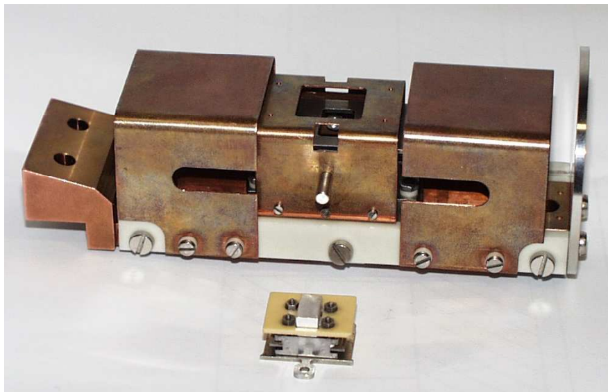
Figure 2.3: A heating type sample holder together with the shielded head of the manipulator are shown. The central shield can be slid laterally to insert the sample plate and to directly access the surface during sample preparation. The sliding is done by means of a wobble stick that grabs the central protruding pin.
