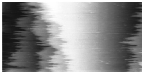
FIG. 1. STM image of the clean Ag(110) surface at 300 K with fluctuating steps ( 340 \times 180 \text{ \AA}^2 , V = -0.5 \text{ V} , I = 0.1 \text{ nA} ).
