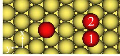
**Fig. 1.** Structures of the investigated systems: the cluster atoms occupy ideal lattice sites of the underlying Pt(111) substrate.
