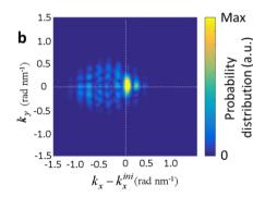
Fig. 1. (a) space-time representation of the electron wavefunction interacting with a silicon grating. The grating is illuminated with light with the electric field amplitude of  $1 \times 10^8$  V/m. Scale bar is 200 nm. (b) The final distribution of the electron wavefunction in momentum space.
