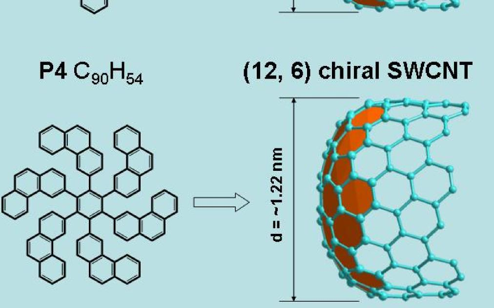
Four precursor molecules for single-wall carbon nanotube end - caps were synthesized. P1 and P2 contain 3 of the required 6 pentagons in their precursor structure while the remaining 3 have to be formed during condensation to the CNT end-cap (step 3 of the growth scenario). For P3 and P4 all 6 pentagons must be formed during the condensation step.
