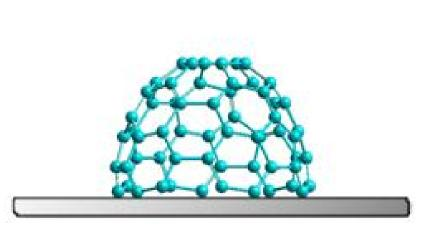
4. Chemical vapor deposition growth of CNT end-caps to full SWCNTs of specific chirality
