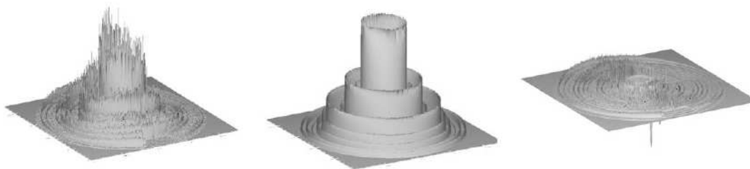
Figure 82: Whole image refinement. The observed intensities ( I_{obs} ) are shown in the left image. In the central image the simulated intensities ( I_{calc} ) are shown. The difference is shown on the right. The calibration parameters are refined to minimize the difference between I_{obs} and I_{calc} .
