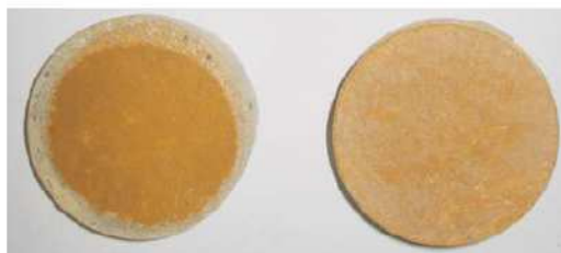
Figure 29: Core drill samples of a yellow magnesia floor from southern Germany. The yellow colour was achieved by mixing iron oxides into the \text{MgO} powder. Left: Correctly colored sample. Right: Bleached sample.
