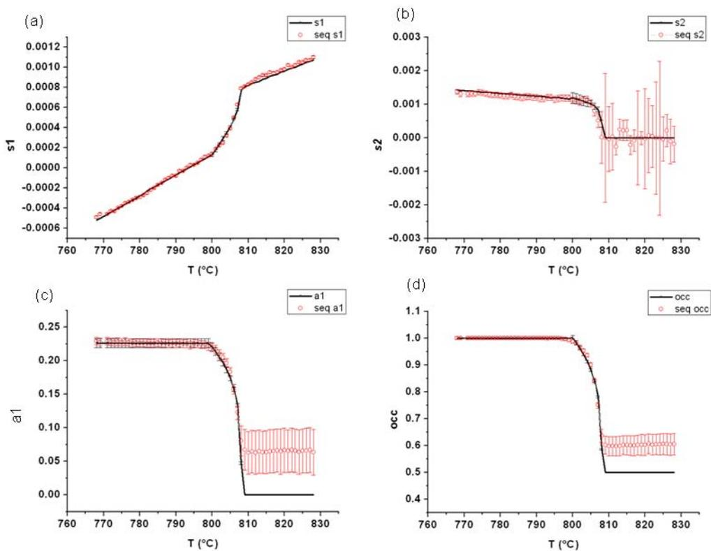
Figure 2: Comparison of values obtained in the parametric (black line) and sequential (red circles) Rietveld refinements. (a) Values obtained for  $s1$  show very good agreement for the whole temperature range. (b) Values for  $s2$  parameter and respective esd's (c) the  $a1$  parameter shows good agreement in the low temperature and transition region (d) Values for the occupancy of Wyckoff position 4a ( $I\bar{4}2d$ ) with copper.
