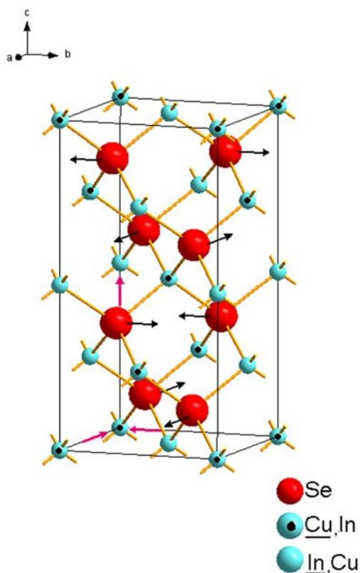
Figure 1: Crystal structure of tetragonal CuInSe<sub>2</sub>. The pink arrows indicate the directions of the tetragonal distortion; the black arrows indicate the movement of the selenium atoms (red). The two different cation positions are given by blue atoms. Cation position 1 (Wyckoff position 4a;  $\bar{4}2d$ ) ((blue atom with black dot) is preferred by copper, while cation position 2 (Wyckoff position 4b;  $\bar{4}2d$ ) (blue atoms) is preferred by indium in the low symmetry phase).
