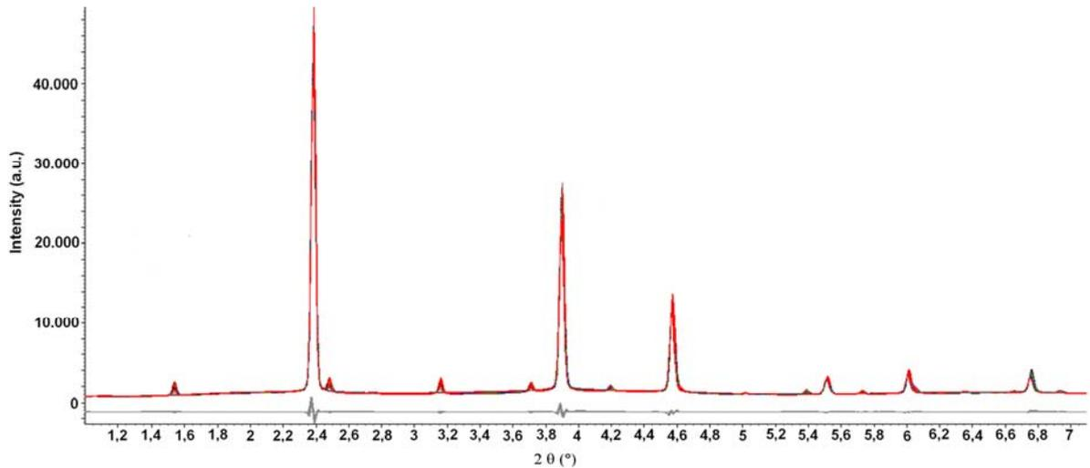
Figure 2: Plot of the parametric Rietveld refinement of the phase transition of CuInSe<sub>2</sub> in the temperature range from 786 °C to 828 °C. Observed and calculated intensities and their differences are plotted for all temperature in steps of 1 °C.
