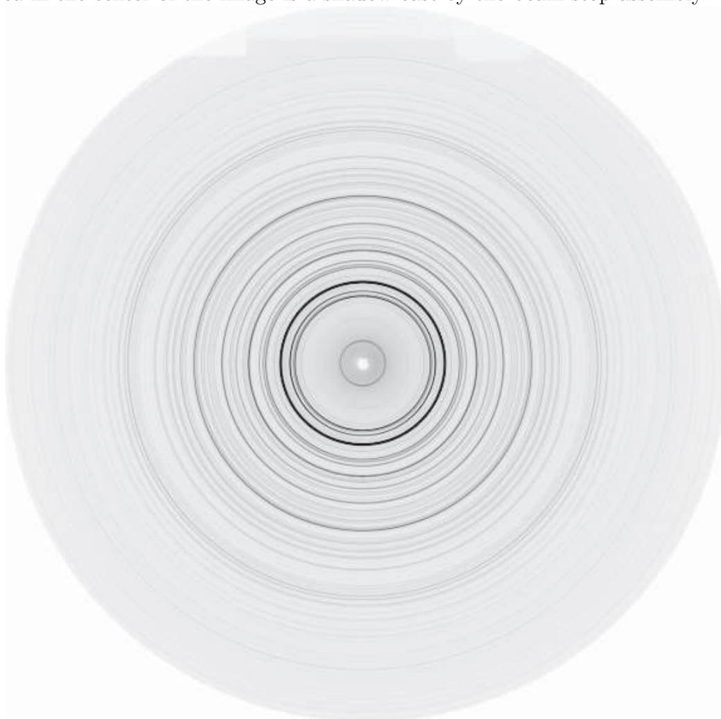
Figure 3.2: X-ray powder diffraction data of  $\text{In}_x\text{Nb}_3\text{Te}_4$  at 0.26 GPa, recorded on a MAR3450 imaging plate detector. The sample was contained in a diamond anvil cell (irradiated volume  $0.001 \text{ mm}^3$ ). The wavelength of the radiation was  $0.43133 \text{ \AA}$ . The white area in the center of the image is a shadow cast by the beam stop assembly.
