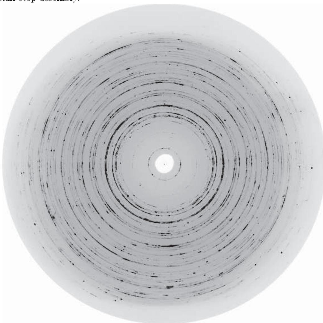
Figure 3.3: X-ray powder diffraction data of  $\text{Nb}_3\text{Te}_4$  at 0.495 GPa, recorded with an online image plate detector (Thoms et al., 1998). The sample was contained in a diamond anvil cell. The wavelength of the radiation was  $0.37380 \text{ \AA}$ . The vertical streak, about 2 cm right of the left edge of the image may be due to a change of the sensitivity of the detector. The light gray area in the top left quadrant of the image is a shadow cast by the beam stop assembly.
