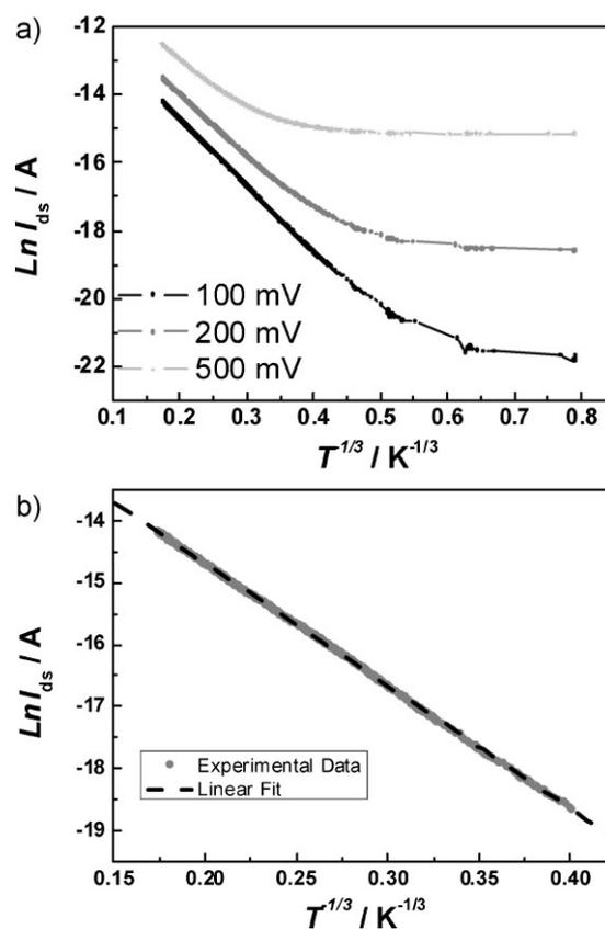
**Figure 4.** Plot of drain–source current ( $I_{ds}$ ) against  $T^{-1/3}$  at different  $V_{ds}$  applied to a CVDGO monolayer. Two regimes of conduction are observed. b) Magnified view of the hopping regime at low bias (100 mV). A two-dimensional variable range hopping model shows a perfect linear fit, indicating the presence of charge transport barriers due to defects.
