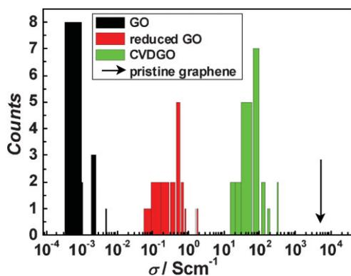
**Figure 1.** Histogram of the experimentally determined electrical conductivity distribution for monolayers of GO, reduced GO and CVDGO. The conductivity of pristine graphene, as reported in the literature [3], has been added for comparison.
