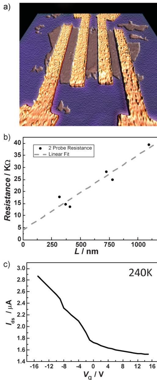
**Figure 2.** a) AFM image of a four-probe CVDGO single-layer device. The scale bar is 1 μm. b) Room-temperature two-probe resistance as a function of channel length measured on the device in the upper panel. The resistance increases linearly with channel length with an intercept at 4 kΩ indicative of the contact resistance. c) Drain-source current as a function of back gate voltage for a device measured at 240 K under a low pressure of helium.
