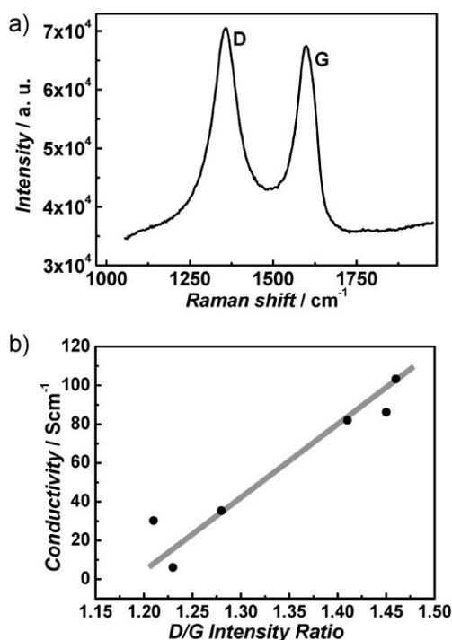
**Figure 3.** a) Representative Raman spectrum of a CVDGO monolayer displaying a D/G ratio larger than 1. b) Plot of conductivity vs. D/G intensity ratio displaying a monotonic rise with conductivity.
