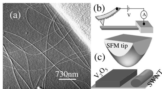
**Figure 1.** Experimental set-up: (a) region of SiO<sub>2</sub> with a gold electrode and a random population of V<sub>2</sub>O<sub>5</sub> nanofibres connected to the electrode. (b) Experimental procedure. (c) Comparison of V<sub>2</sub>O<sub>5</sub> nanofibres with other cylindrical molecules.
