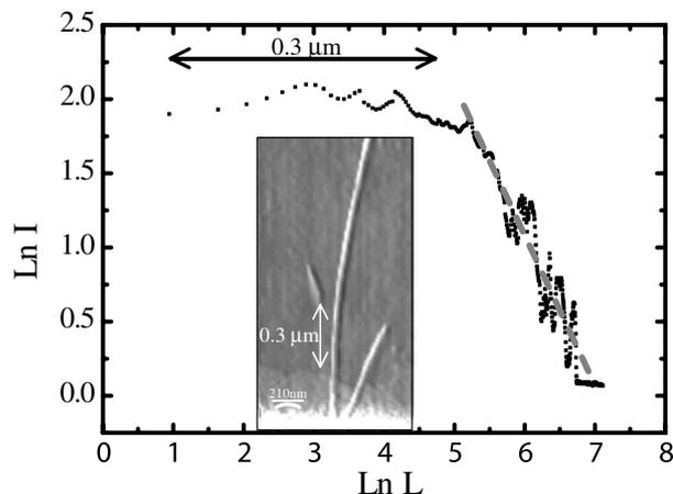
**Figure 4.** In the inset, the topographic image of a  $V_2O_5$  nanofibre connected to a gold electrode is shown. The chart represents the log-log plot of the current versus length for the longest fibre of the inset. A linear behaviour with slope  $-1.01$  is found for  $L > 300$  nm ( $E < 1.3 \times 10^{-5}$  V  $cm^{-1}$ ); for lower values of  $L$  the dependence is weaker due to a higher conductivity than that expected for an ohmic conductor.
