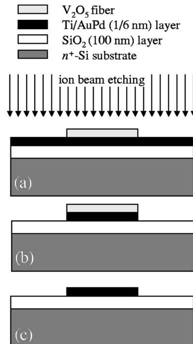
FIG. 1. Schematic illustration of the nanowire fabrication process. (a)  $V_2O_5$  fibers are employed as an etching mask on top of the thin metal layer. (b) AuPd film unprotected by the etching mask is removed by IBE. (c) Remaining parts of the  $V_2O_5$  wires are removed with a dilute acid solution.
