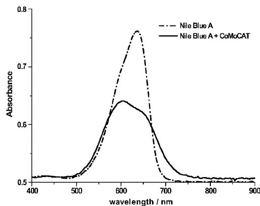
**Figure 5.** Absorption spectra of  $3.0 \mu\text{m}$  (final concentration) Nile blue A in the absence and presence of CoMoCAT nanotubes. The absence of a redshift signifies that the quenching of Nile blue A is dynamic in nature.
