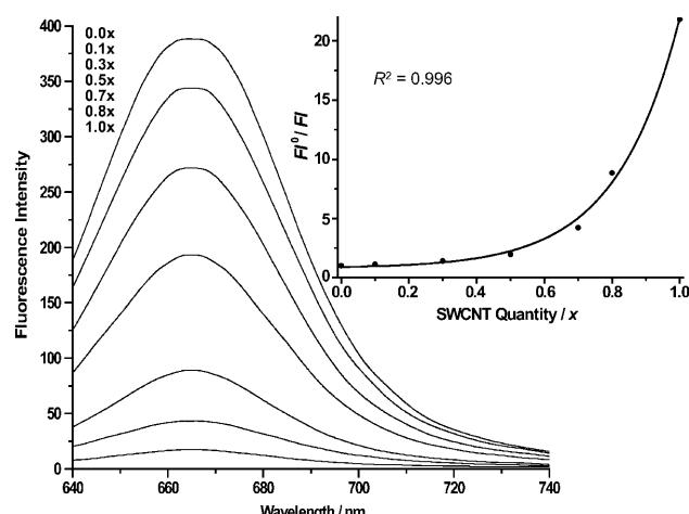
**Figure 2.** The emission spectrum of 2.5  $\mu\text{M}$  (final concentration) Nile blue A in the presence of different CoMoCAT nanotube concentrations (excitation wavelength: 635 nm). 1x refers to the starting concentration after centrifugation. The inset is a Stern–Volmer plot showing the ratio of the emission intensity (at 665 nm) in the absence of nanotubes ( $F^0$ ) to the intensity in the presence of nanotubes ( $F$ ).
