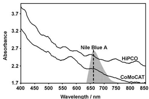
**Figure 3.** Optical absorption spectra of CoMoCAT and HiPCO SWCNTs (1x in both cases). The shaded areas show the emission spectrum of Nile blue A, indicating the spectral overlap with the second van Hove energy ( $E_{22}^S$ ) of the SWCNTs in the respective samples. The dashed line represents the wavelength of the emission maximum for Nile blue A (665 nm).
