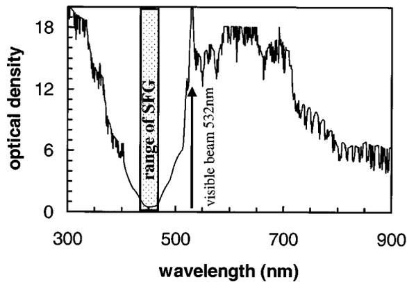
FIG. 3. Synthetic absorption curve of the four-filter-combination discussed in the text. The curve is the product of four absorbance curves measured for the individual filters. Due to the limited sensitivity of the spectrometer optical densities larger than five may be underestimated in this plot and may in reality be larger.
