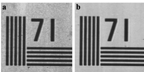
FIG. 4. Examples of the reduction of grating and filter inhomogeneities: (a) raw image; (b) the same image after normalization to an average of blank images (also see the text).
