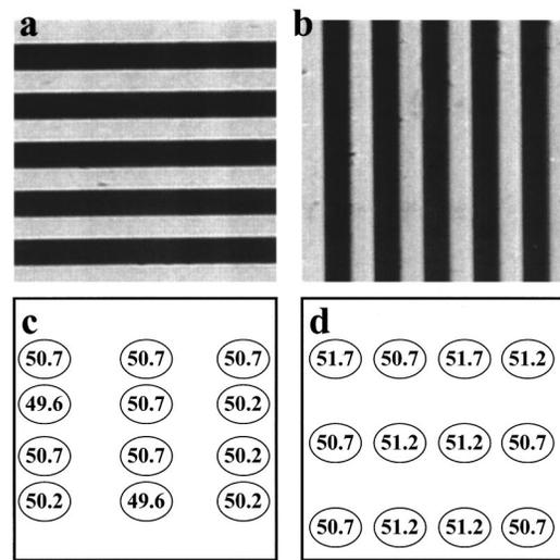
FIG. 5. Determination of image distortion. Top: image of a 22 linepairs/mm structure (a) for horizontal lines; (b) for vertical lines. Bottom: values obtained by evaluating the magnification in different parts of the images (c) for the vertical magnification; (d) for the horizontal magnification. The magnification values are printed in the region of the box equivalent to the region where they have been obtained in images (a) and (b).
