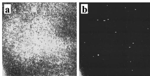
FIG. 7. Proof of background suppression: Uncorrected raw data with 5 min exposure time,  $4 \times 4$  pixels binned. (a) SFG intensity from a GaAs sample; (b) same conditions but with the visible beam delayed by 50 ps with respect to the IR beam. The intensity scales for both images are identical. White pixels in (b) are due to cosmic rays. The bright spot in the lower left corner is due to an inhomogeneity of CCD dark current.
