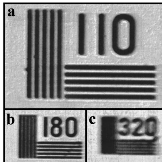
FIG. 6. (a) Well-resolved test pattern (110 linepairs/mm); (b) resolution limit for vertical lines: 180 line pairs/mm; (c) for horizontal lines: 320 line pairs/mm.
