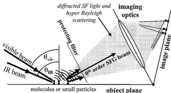
FIG. 1. Principle of SFG microscopy. In contrast to “classical” SFG spectroscopy not only the specular beam is observed. Diffracted beams contain the light emitted by pointlike sources and carry the information of sample inhomogeneities.
