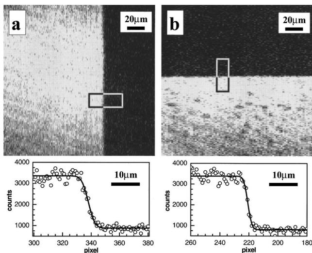
FIG. 8. Resolution in a SFG image: (a) for a vertical and (b) a horizontal edge of a GaAs sample. The exposure time was 120 min. In the measurements, four pixels parallel to the edge were binned keeping the resolution perpendicular to the edges. At the bottom the average of eight line scans in the boxed area are shown together with the fits discussed in the text.
