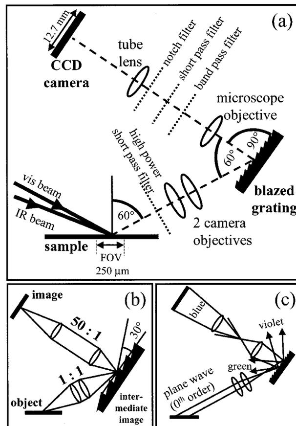
FIG. 2. (a) Schematic setup of the SFG microscope with the employed optical elements. (b) Path of the imaging beam. (c) Path of the illumination beam. FOV=field of view.
