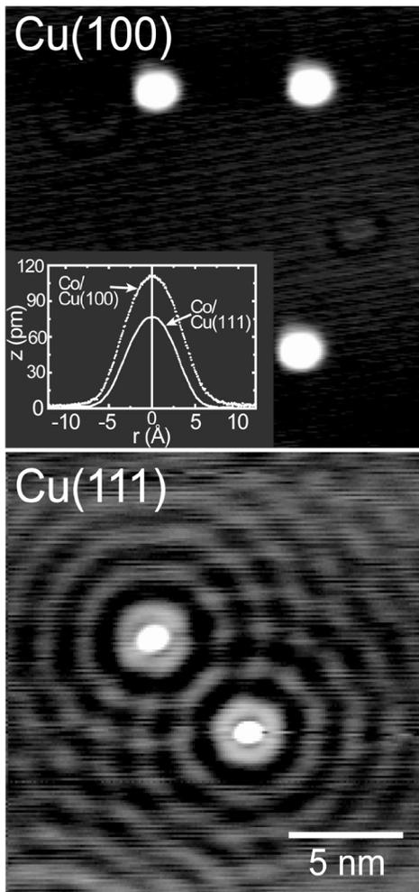
FIG. 1. Constant current STM images ( $-50$  mV bias,  $I = 2$  nA) of Co adatoms on the Cu(100) (three atoms) and the Cu(111) surface (two atoms). The Friedel oscillations of the Cu(111) surface state electrons can be easily detected up to 10 nm. The inset compares line cuts in the  $z$  signal over the adatoms on the two different surfaces for typical tip conditions.
