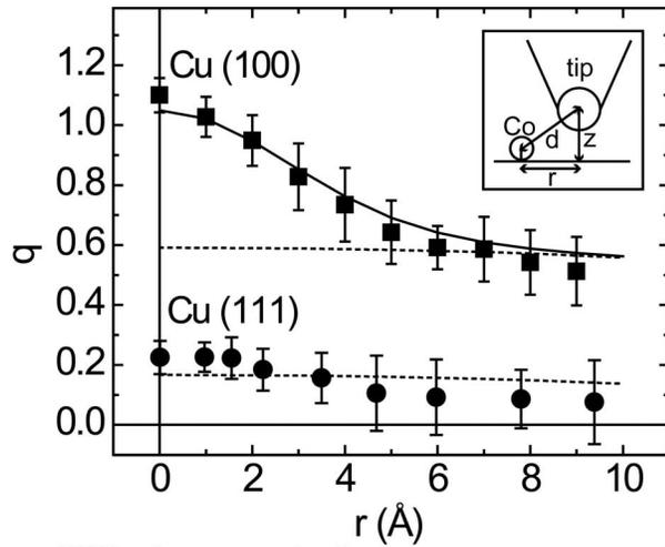
FIG. 3. Spatial dependence of the Fano line shape parameter  $q$  on the in-plane tip-adatom distance  $r$  for Co/Cu(100) and Co/Cu(111). Each data set presents averaged values from measurements on four atoms. The dotted lines are from calculations with no direct tunneling into the localized state, for the solid line  $t(r)$  was fitted as described in the text. The inset shows the measurement geometry.
