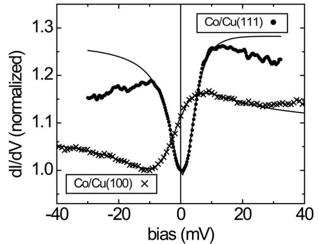
FIG. 2. Atom differential conductance ( $dI/dV$ ) spectra for Co/Cu(100) and Co/Cu(111). The tunneling resistance was  $10$  M $\Omega$ . The spectra are normalized to their lowest values. The solid lines are Fano line shape fits according to Eq. (1); average parameters are summarized in Table I.
