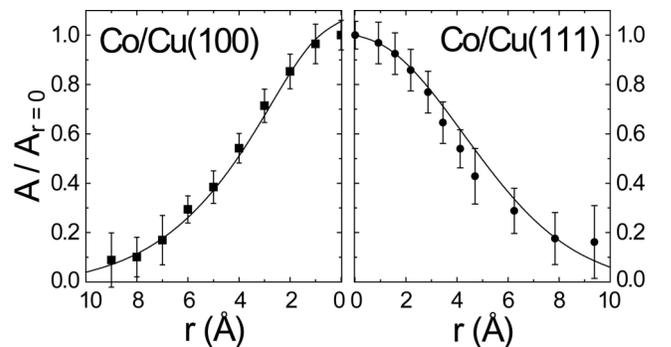
FIG. 4. Spatial dependence of the normalized amplitude of the Fano resonance  $A(r)/A(0)$  on the in-plane tip-adatom distance  $r$  for Co/Cu(100) and Co/Cu(111). Each data set presents averaged values from measurements on four atoms. The solid lines are from model calculations described in the text.
