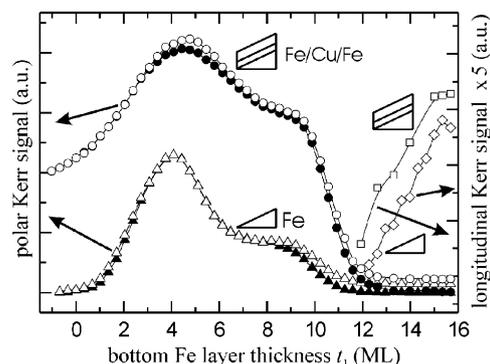
Fig. 1. Polar remanent ( $\blacktriangle$ ), polar saturation ( $\triangle$ ) and longitudinal saturation ( $\diamond$ ) Kerr intensity of MOKE loops of a Fe wedge on Cu(100) as a function of Fe thickness,  $t_1$ , taken at  $T = 200 \text{ K}$ . Polar remanent ( $\bullet$ ), polar saturation ( $\circ$ ) and longitudinal saturation ( $\square$ ) Kerr intensity of MOKE loops of a trilayer, 3 ML Fe/2 ML Cu/ $t_1$  ML Fe, as a function of the bottom Fe layer thickness,  $t_1$ , taken at 90 K.
