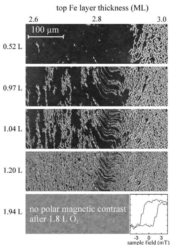
Fig. 3. Kerr images of the remanent state of  $t_2$  ML Fe/2 ML Cu/3 ML Fe captured during oxygen adsorption at 125 K. Inset: longitudinal MOKE loop of the trilayer taken after the adsorption of 1.94 L  $O_2$ . Image size:  $400 \mu\text{m} \times 110 \mu\text{m}$ .
