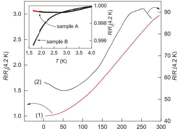
Figure 2: Temperature dependence of the magnetoresistance before (1) and after (2) application of a current pulse of  $\approx 10^5$  A/cm<sup>2</sup>. Low temperature resistances of two different samples are shown in the inset.
