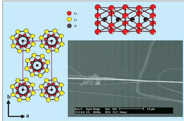
Figure 1: Left: Projection of the crystal structure of Ta<sub>4</sub>Te<sub>4</sub>Si along [001]. Right top: Part of an infinite Ta-Si strand extending along [001]. Right bottom: Electron microscope graph of Ta<sub>4</sub>Te<sub>4</sub>Si fibers.
