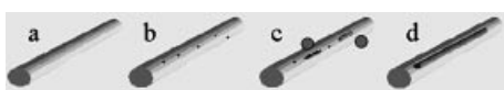
Figure 11. Mechanism of electroless cluster and wire deposition inside a channel: (a) tube-like template (e.g. TMV); (b) sensitisation: formation of very small noble metal clusters on the exterior surface and on the interior walls; (c) initial deposition: only a few very active clusters grow fast, the clusters on the exterior surface detach; (d) the clusters inside the channel can grow to, at maximum, two wires per channel when metal ions are supplied from the orifices of the channel.
