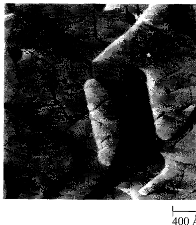
Fig. 1. Morphology of a Au(111) surface covered by a decanethiol self-assembled monolayer. After self-assembly the surface has been annealed for three hours at 360 K. The image size is 3000 \text{ \AA} \times 3000 \text{ \AA} .
