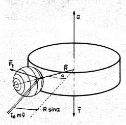
Fig. 1 Freely rotating disk as momentum flux detector α-angle of incidence, ω-angular velocity, R- disk radius, P<sub>t</sub>- the tangential force, f-the resulting torque.
