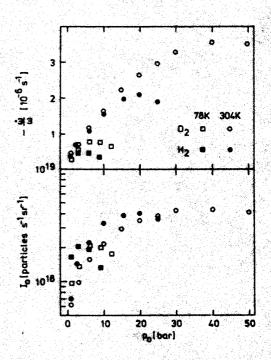
Fig. 4 The measured rotor decelerations (-u/w) due to the impinging beam particles and the resulting absolute intensity date as a function of the stagnation pressure at stagnation temperatures of 18 % and 304 K.
