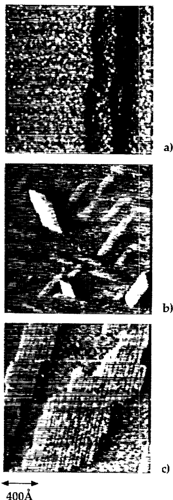
Fig. 2. The growth of palladium silicide on Pd(110) at 300 K (a), at 400 K (b) and at 550 K (c). The Si deposition at the surface is 0.4 ML.
