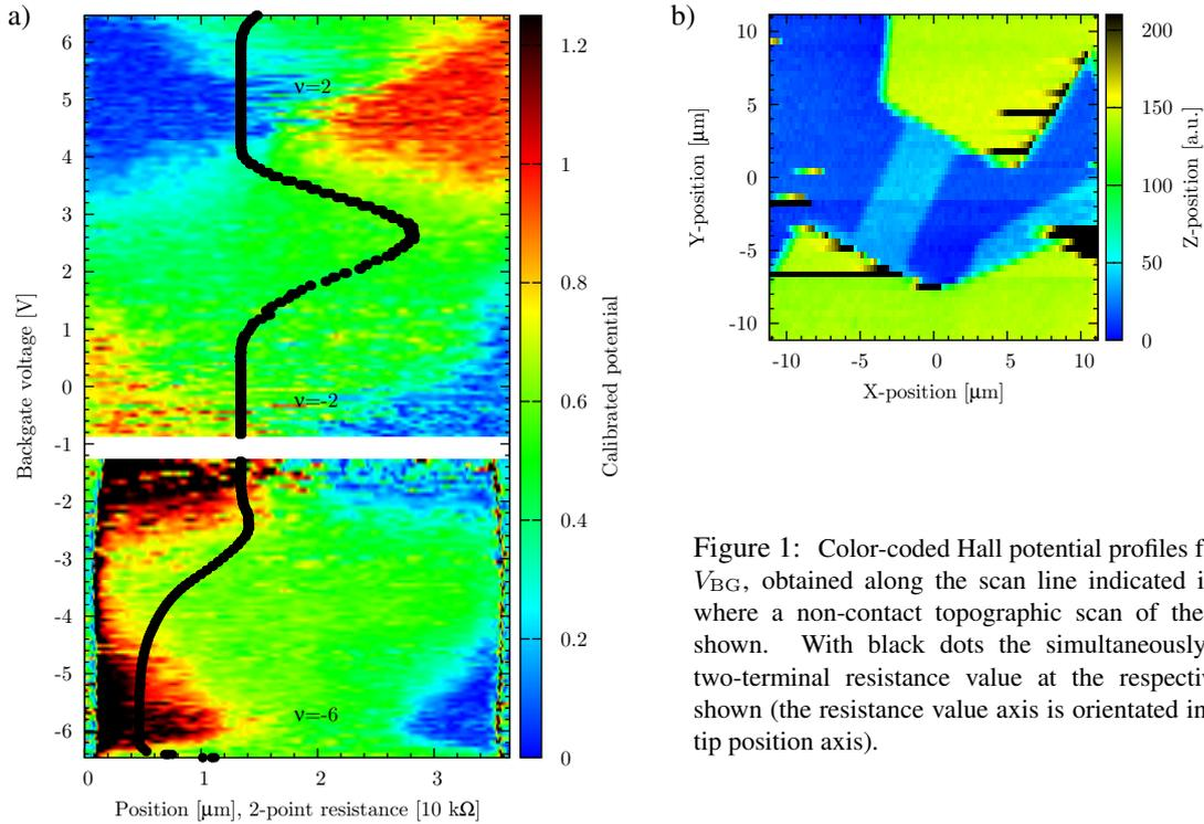
Figure 1: Color-coded Hall potential profiles for different  $V_{BG}$ , obtained along the scan line indicated in the inset where a non-contact topographic scan of the sample is shown. With black dots the simultaneously measured two-terminal resistance value at the respective  $V_{BG}$  is shown (the resistance value axis is orientated in parallel to tip position axis).
