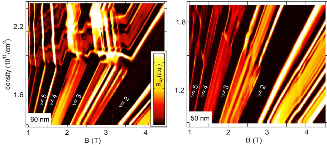
Figure 2: Longitudinal resistance. (a) In the 60 nm sample, when two subbands are populated their quantum Hall features coexist. In particular, a quantized  $5/2$  state of the lower subband is observed even when the second subband is populated. (b) In the 50 nm sample the quantum Hall features follow the total density.
