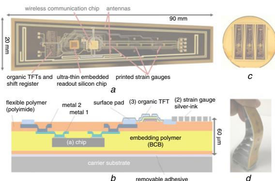
**Fig. 1** The hybrid system-in-foil technology
