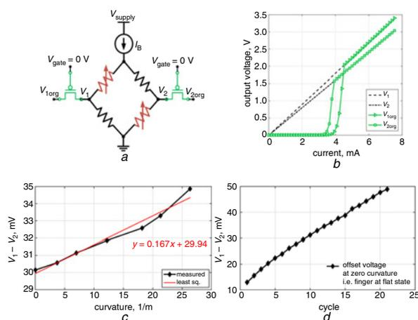
**Fig. 3** Characterization of the printed strain gauge and organic TFT switch
