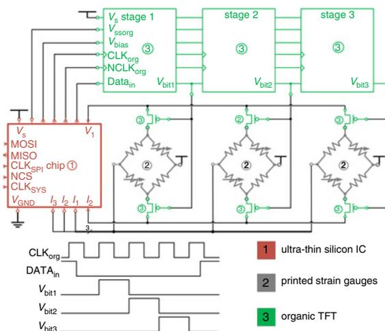
**Fig. 2** Schematic of main HySiF component parts. It includes three printed strain gauges, three-stage organic shift register, three pairs of organic TFT switches and ultra-thin silicon readout chip
