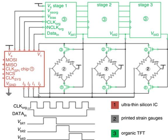
**Fig. 2** Schematic of main HySiF component parts. It includes three printed strain gauges, three-stage organic shift register, three pairs of organic TFT switches and ultra-thin silicon readout chip
