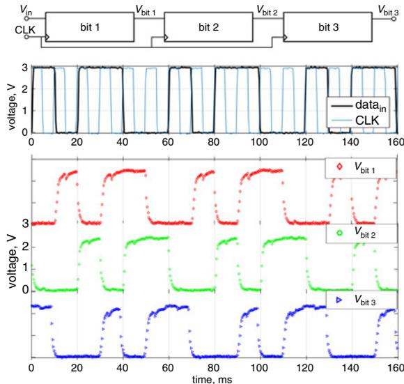
**Fig. 4** Schematic and measurements of three-stage shift register, which is based on dynamic positive-edge-trigger master-slave flip-flop using biased-load inverters
