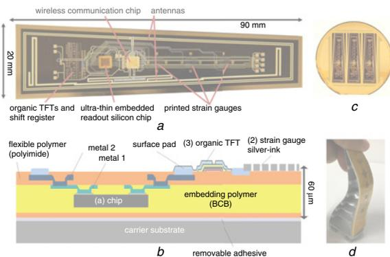
**Fig. 1** The hybrid system-in-foil technology
