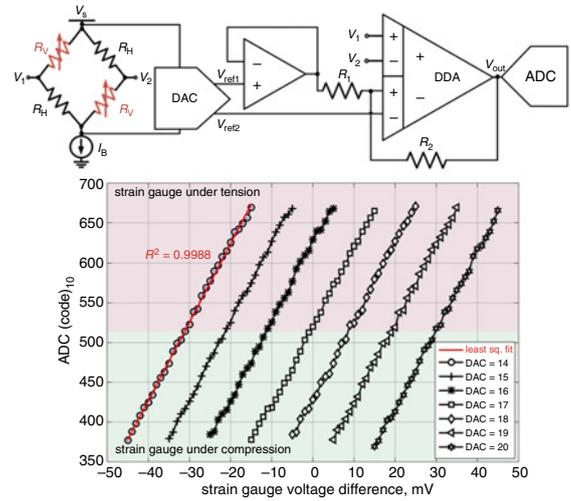
**Fig. 5** Schematic and measurement results of the sensor readout circuit implemented in ultra-thin silicon chip at different offset cancellation voltages
