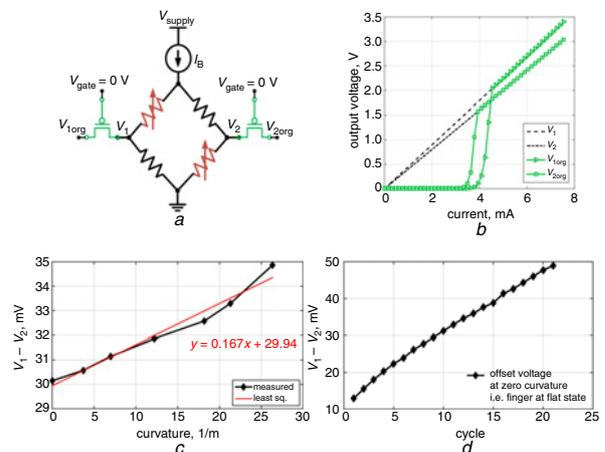
**Fig. 3** Characterization of the printed strain gauge and organic TFT switch
