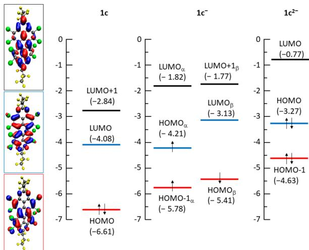
**Figure 4.** Molecular frontier orbitals of neutral, monoanionic, and dianionic compound **1c** and their orbital energies in eV, calculated at B3LYP/TZVPP level of theory employing COSMO.
