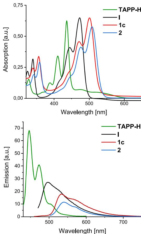
**Figure 2.** Absorption (top) and emission spectra (bottom) of fully halogenated TAPPs in THF ( $c = (1.2\text{--}1.6) \times 10^{-5}$  M), compared to the bay-chlorinated (I) and unsubstituted (TAPP-H) TAPPs.
