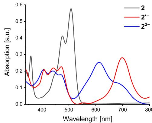
**Figure 3.** Absorption spectra of **2** and the corresponding monoanion  $2^{\bullet-}$  and dianion  $2^{2-}$  measured in THF ( $c = 1.2 \times 10^{-5}$  M).
