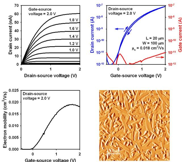
**Electrical characteristics of n-channel organic thin-film transistors with a vacuum-deposited layer of **1** as the semiconductor measured in ambient air, and AFM image of the organic-semiconductor surface.**
