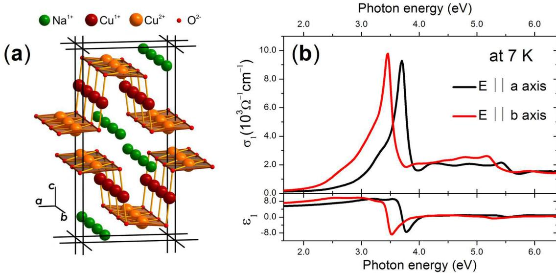
Figure 1: (a) Crystal structure of  $\text{NaCu}_2\text{O}_2$ . (b) Real part  $\epsilon_1$  of the dielectric function and real part  $\sigma_1$  of the optical conductivity of  $\text{NaCu}_2\text{O}_2$  measured at 7K for polarizations along ( $E \parallel b$ ) and perpendicular ( $E \parallel a$ ) to the  $\text{Cu}^{2+}\text{O}_4^{2-}$  chains.
