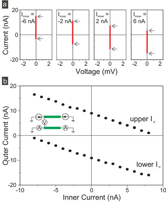
Figure 2: (a) Tunneling current-voltage characteristics of the outer contacts with different constant currents passing through the inner contacts. The critical currents through the outer contacts are increased (decreased) if an additional current flows through the inner contacts in the opposite (same) direction. (b) Upper and lower (positive and negative) critical currents measured at the outer contacts as function of the Josephson current passing through the inner ones (black dots).
