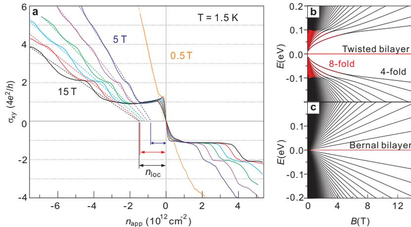
Figure 2: (a) Hall conductivity as a function of  $n_{\text{app}}$ . (b-c) LL spectra of (b) twisted bilayer graphene and of (c) Bernal stacked bilayer graphene. The degeneracy of the energy levels is color coded: red corresponds to 8-fold degenerate and black to 4-fold degenerate.
