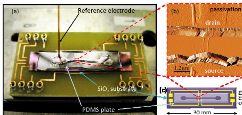
Figure 1: DNA biosensor based on CNTs. (a) Photograph showing the chip carrier with the sensor chip covered with a polydimethylsiloxane (PDMS) microchannel containing a test solution. (b) AFM image of the sensor area showing CNTs trapped between two electrodes. (c) Schematic illustration of the sensor chip showing lead electrodes, the electrode gap and the microchannel.
